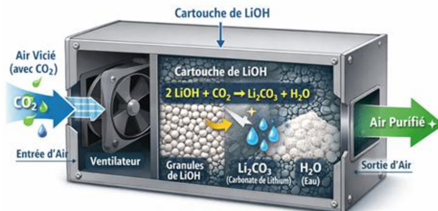
Figure 2: LiOH-Based \text{CO}_2 Removal System
