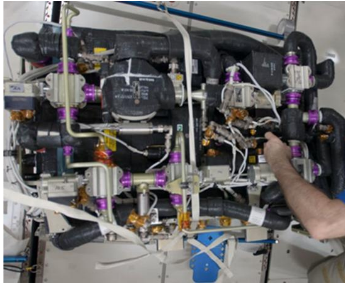
Figure 6: CDRA maintenance onboard ISS.
