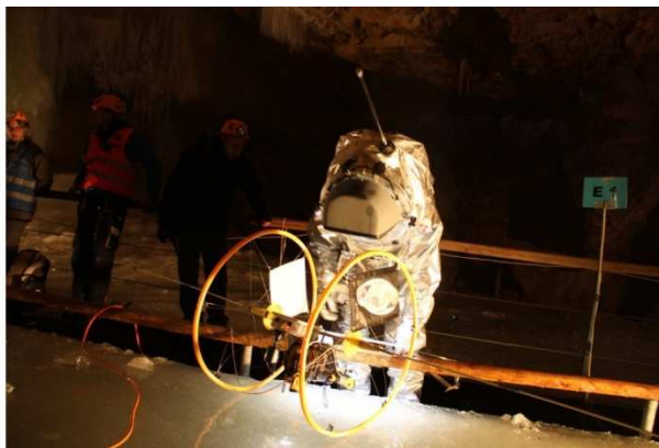
12.15.15 (left): left flashlight set on; the emitter box is on from the position of the two switches. The camera container is open.
