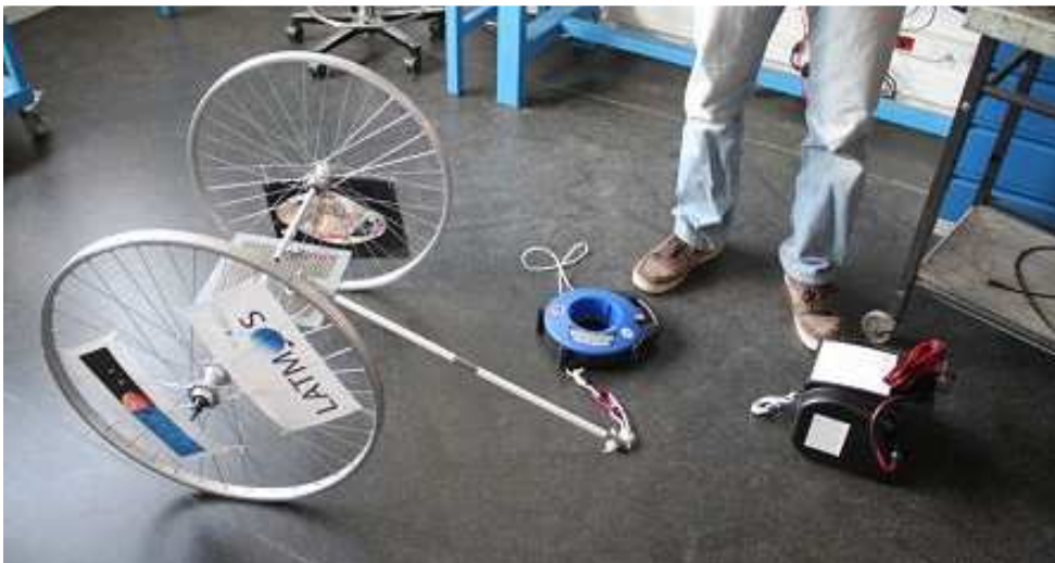
The CRV 5 as delivered to Latmos. The Latmos team changed the instrument plate and added tubes on the wheels. The anti yaw rod and rope were replaced by the cable associated with the electric winch which is on the right of the picture.
