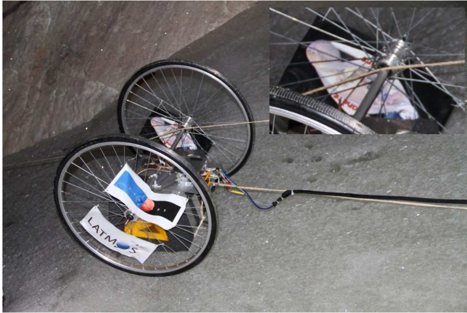
Close view of the CRV 5 with the Exomars ground sounding radar antennas in yellow with black foam protection around. The signal is sent by the black wire linked to the main rope. The association Planète Mars logo is on the right wheel.
