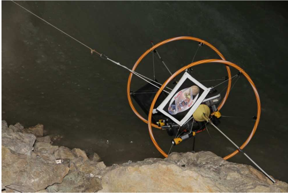
The repair configuration with transition from one to two ropes after the rod attachment failure the day before is visible there.
