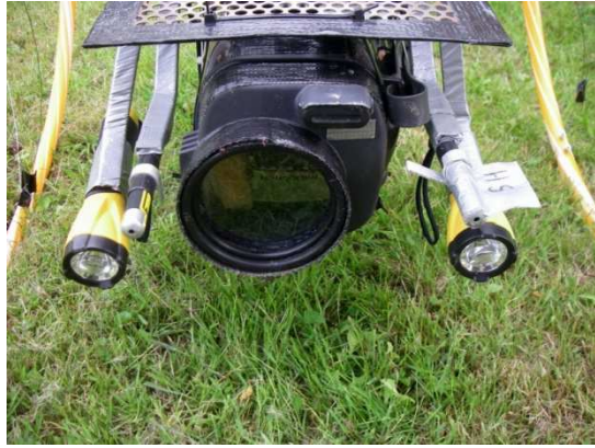
On the left: rear side with the renewed porthole on the camera container, the two flashlights and the two lasers. On the right zoom on the lasers and flashlight.
