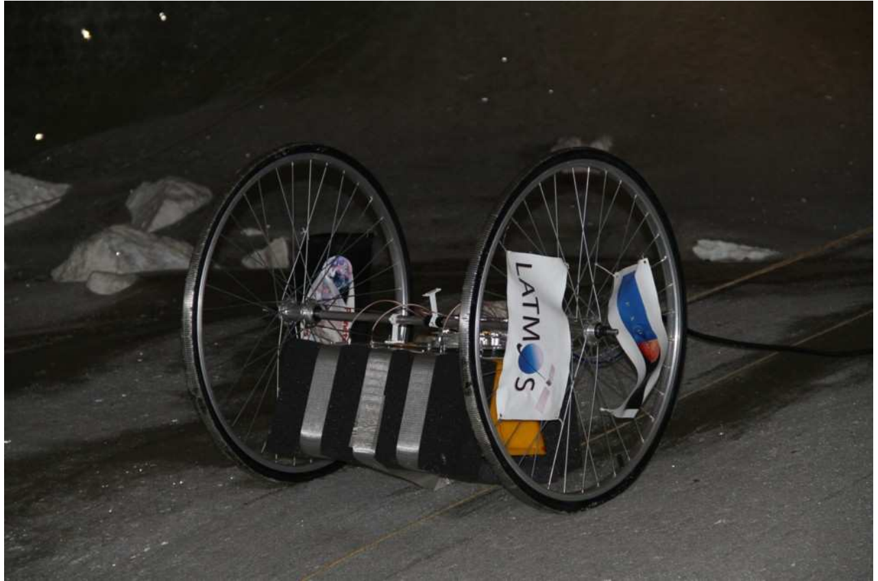
The CRV 5 from front side with the foam protected antennas (and on the wheel on the left the Association Planète Mars logo)
