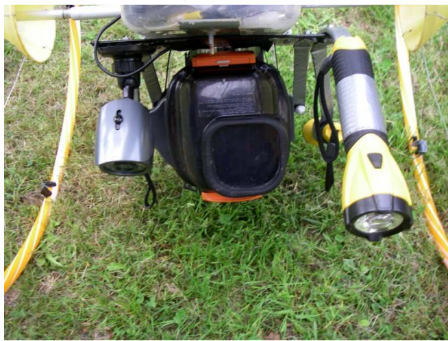
In the left: front side with the hazcam on the left and the flashlight illuminating the hazcam field of view. On the right: the emitter box and its switches.
