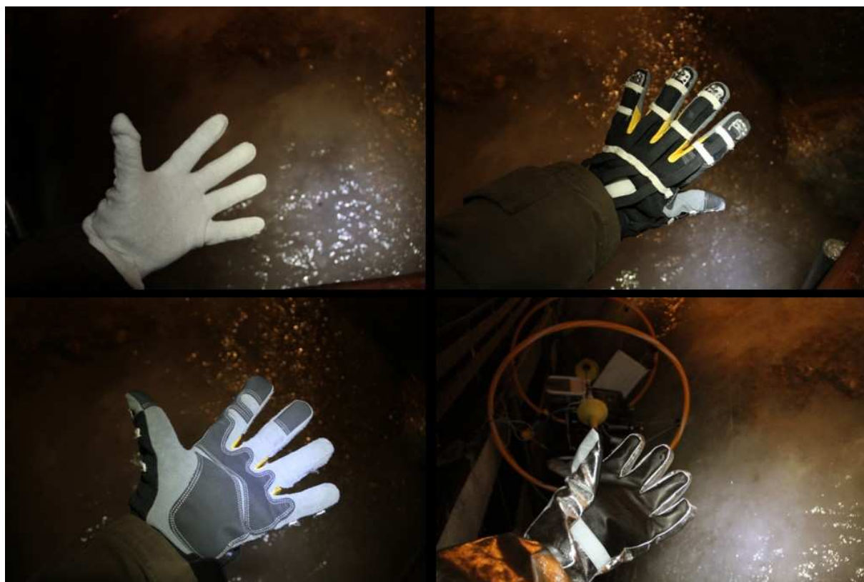
The Aouda three layers of gloves: from left to right and up to down, the comfort glove, the glove restituting the pressure forces from both sides and the outside glove from the palm side.
