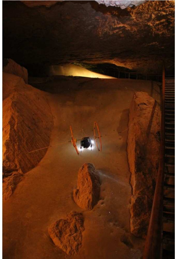
13.07.31 and 13.08.01: rope at 30 m. In the left photo the anti roll rod characteristics are clearly visible: the first half is rigid and the second half flexible. On the other side the anti roll rod fixation has been deformed when the vehicle was stuck behind the rock. On the right photo nearly all the slope is visible. The starting point is on the pathway above the brightly lighted ice bank.
