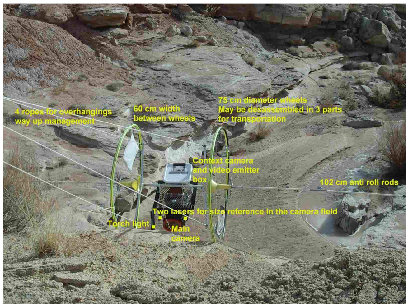
Cliff Reconnaissance Vehicle n°3 main features (CRV test 70 at White Rock Canyon during MDRS 43 in 2006). Small modifications were introduced between this configuration and the CRV 3-3 configuration tested in Dachstein.
