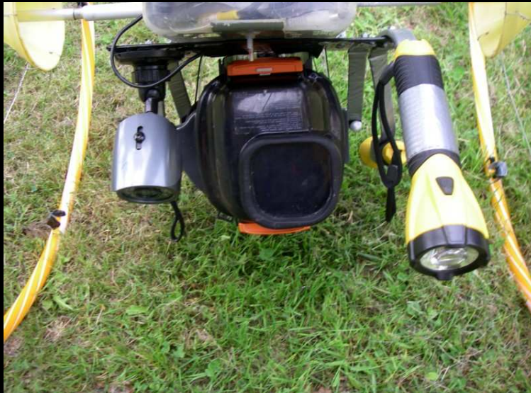
Vehicule front with main camera container cover, new color orientable hazcam (on the left) and flashlighth (on the right) for the hazcam field of view
