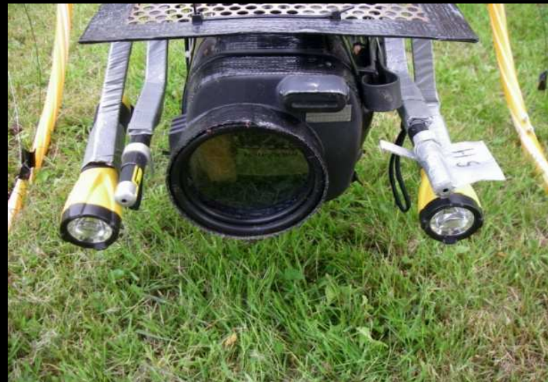
Vehicule front with main camera container cover, new color orientable hazcam (on the left) and flashlighth (on the right) for the hazcam field of view
