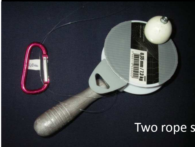
A 250 m thin nylon wire with 1st 50 m doubled Rupture load one wire: 7,5 daN
